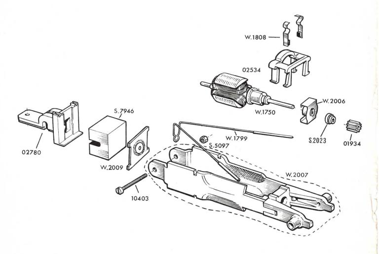
Armature Brush Spring and Insulators Carbon Brush
